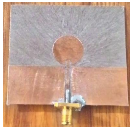
Figure 2. Fabricated CPW fed CMMA on magneto-dielectric substrate
