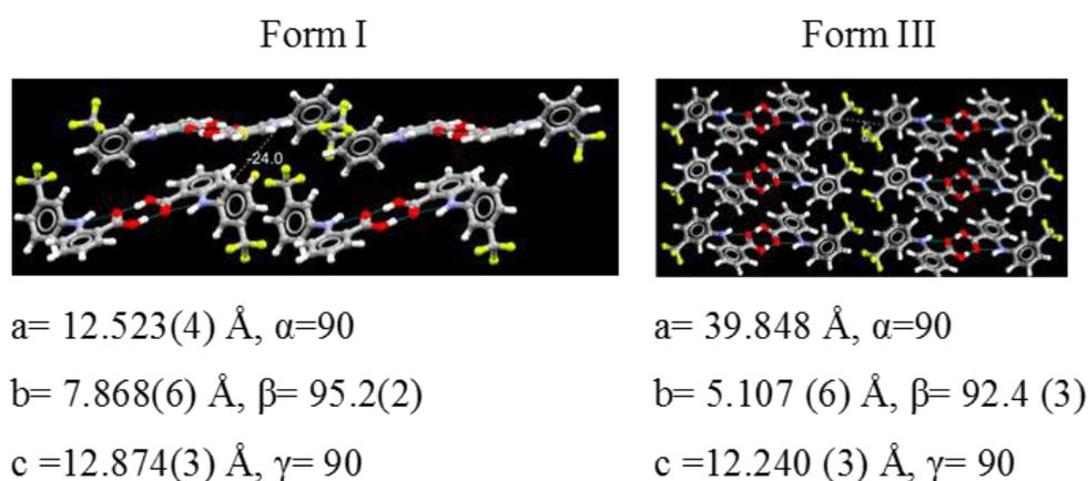
**Figure 2.** Acid $\cdots$ acid heterosynthon via O–H $\cdots$ O hydrogen bonds in the crystal structure of form **I** and form **III**, layered structure guided by weak C–H $\cdots\pi$  interaction in form **I**. A slip-plan along c-axis is prevalent in form **III**.
