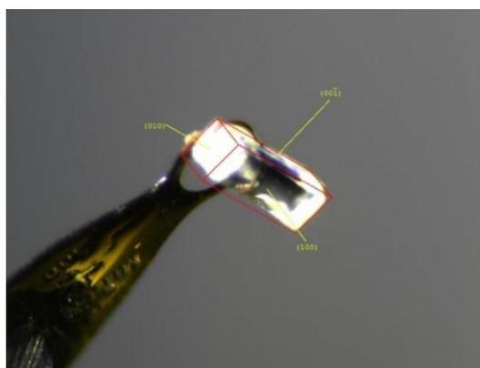
**Figure 4:** Face indexing of polymorph **III** crystal.
