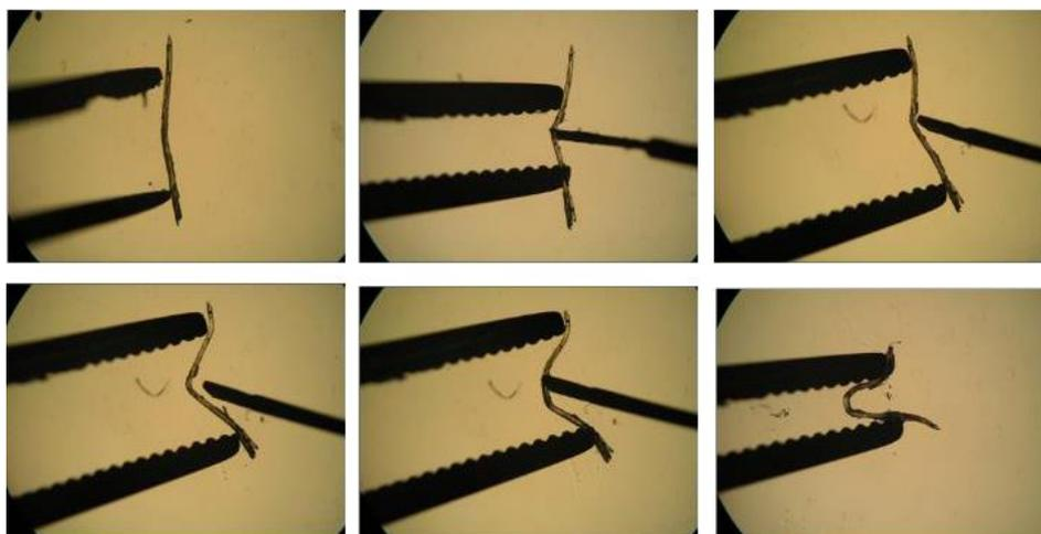
**Figure 3:** Microscopic images (scale bar 200  $\mu\text{m}$ ) demonstrate the plastic bending of polymorph **III** crystals of FA.
