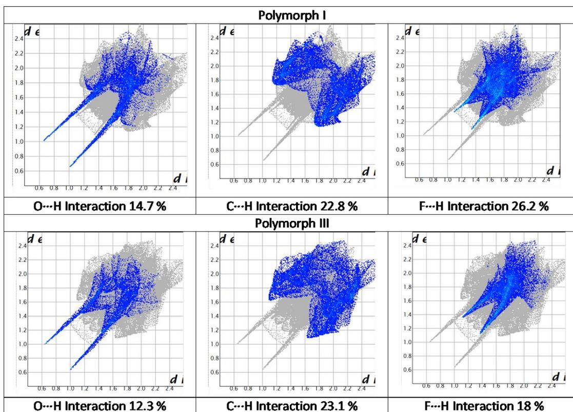
**Figure 5.** Hirshfeld surfaces show high F...H interaction contributions in polymorph I compared to polymorph III leading to brittle behaviour.
